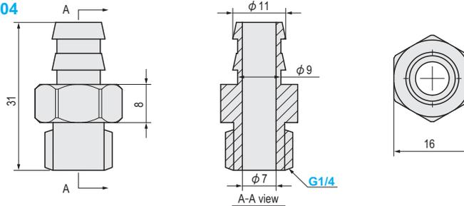
This is used to connect the suction cup and the metal fitting.
