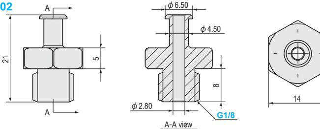
This is used to connect the suction cup and the metal fitting.
