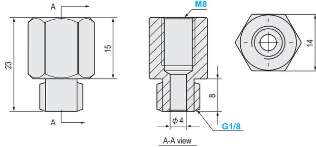
This is used to connect the suction cup and the metal fitting.
