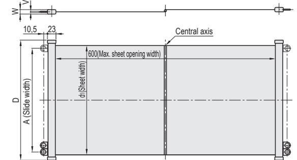
ⓘ M-KSD500 and M-KSD600 have 3 rings on one side for magnet hook.
