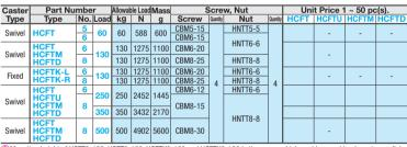
Mounting height of HCFT6-130, HCFT8-130, HCFTK6-130 and HCFTK8-130 is the same, which enables combined use in parallel.
