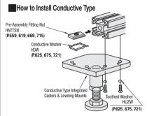
Conductive washers and toothed washers are not included with Conductive Type.
