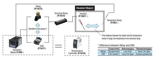
Temperature controller is the unit of a temperature adjuster and SSR.
