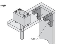
Precision Casting Economy Gussets are optimal for reinforcing where not visible or appearance is not important.
