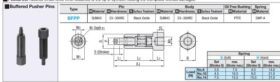
Values of applicable cylinder tube I.D. are for reference. Check for specifications of the cylinder in use.
